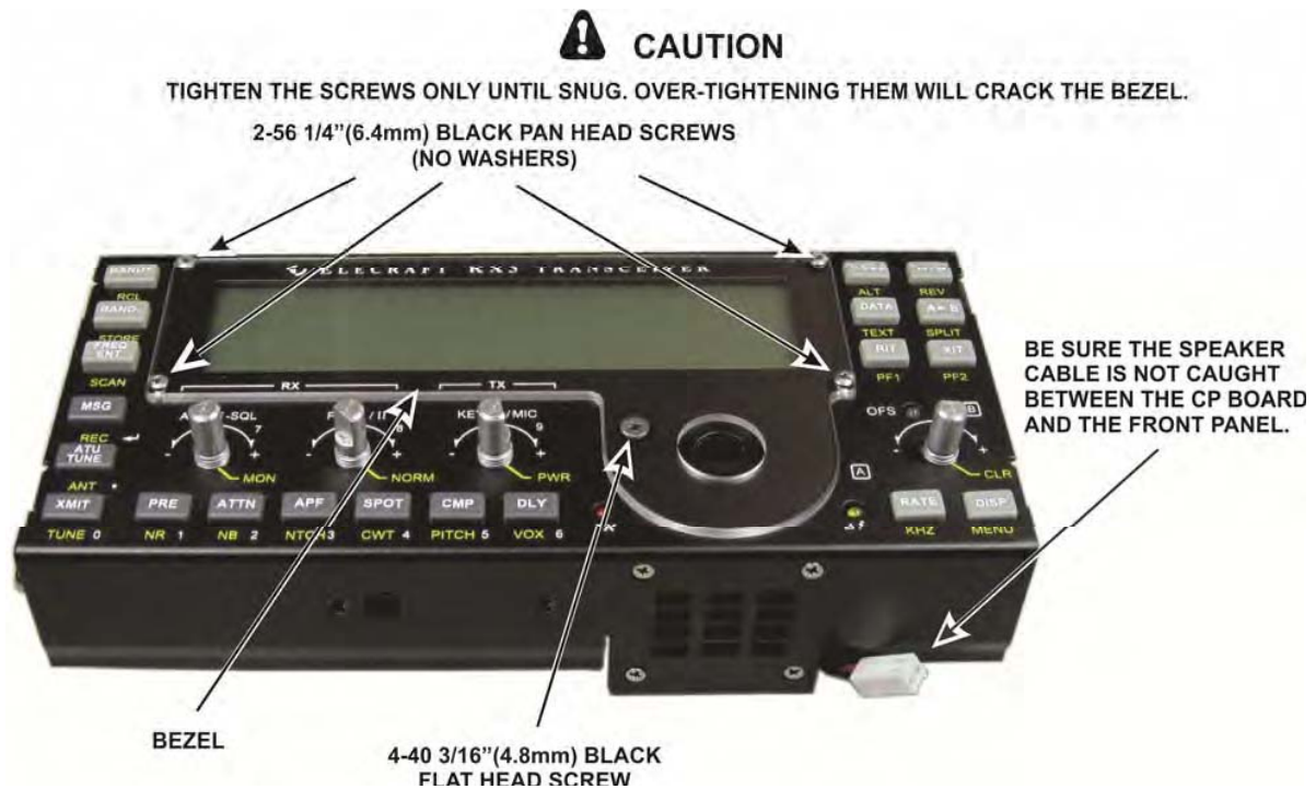
Figure 17. Placing the CP Board in the Front Panel.
