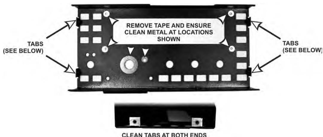
Figure 4. Front Panel Clean Contact Areas.
