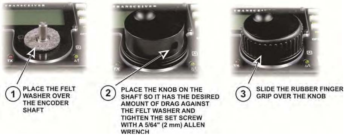
Figure 23. Mounting the VFO Knob.
