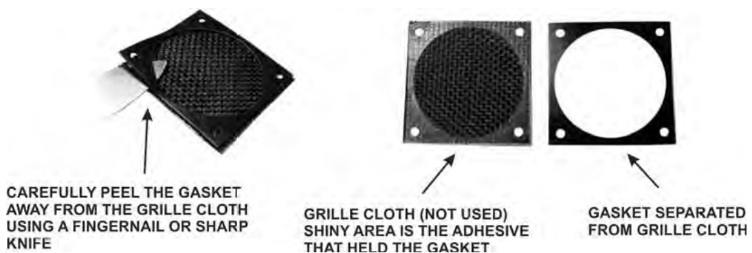
Figure 7. Separating the Gasket from the Grille Cloth.
