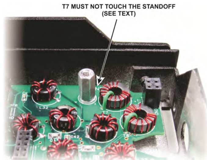
Figure 39. Checking T7 Clearance.
