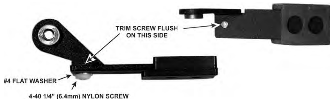
Figure 34. Placing Nylon Bumpers on the Tilt Legs.
